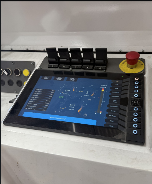
TRIPPING – HOOK LOAD, HOOK POSITION, DEADMAN PROMPT
