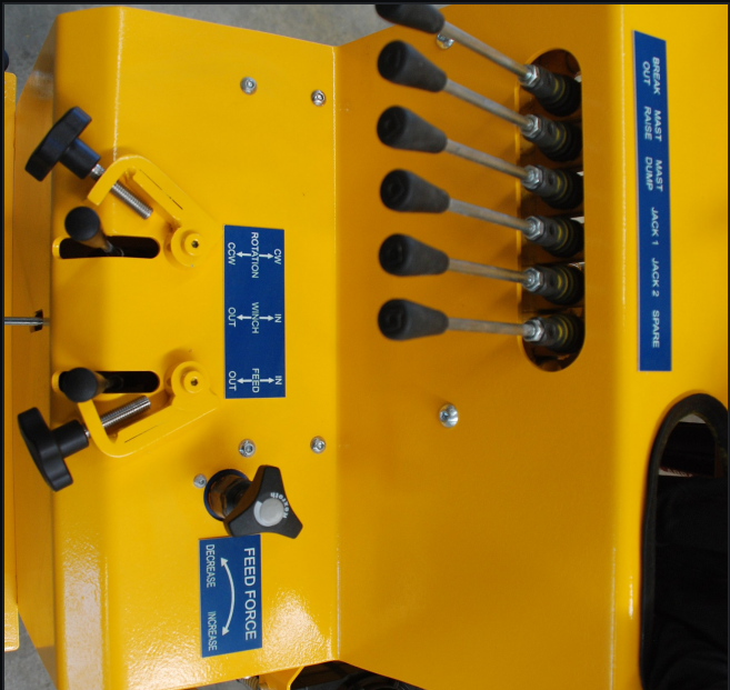
BREAK OUT, MAST RAISE, MAST DUMP, JACKS – ROTATION, WINCH AND FEED ON THE LEVERS, WITH FEED FORCE SET ON THE DIAL
