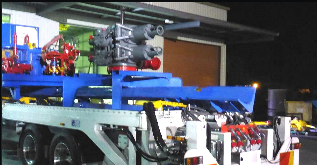
TRANSPORT SKID IN USE – BOP STACK AND TOOL SKID CARRIED ON THE CATWALK BETWEEN WELL SITES, ON CONTAINER TWIST LOCKS
