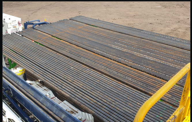
RACK RAILS LOADED – UHMWPE ROLLING EDGES PROTECT THE PIPE
