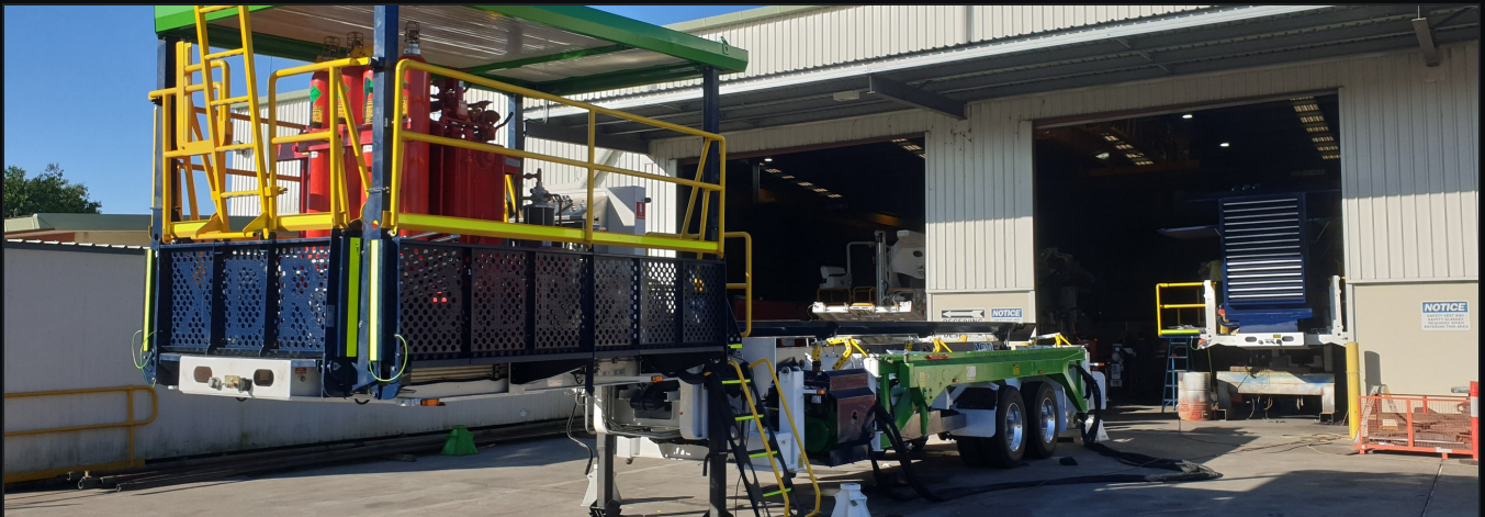
KOOMEY MOUNTING OPTION — CLIENT-SUPPLIED UNIT ON THE GOOSENECK, UNDER THE INTEGRATED ROOF STRUCTURE, WITH 360° ACCESS ON HYDRAULIC PLATFORMS
