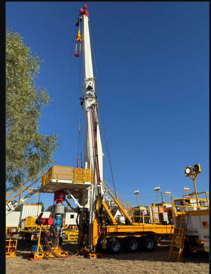
XDR ELECTRIC RIG ON SITE – AUSTRALIAN TWIN PERMANENT-MAGNET VARIANT
