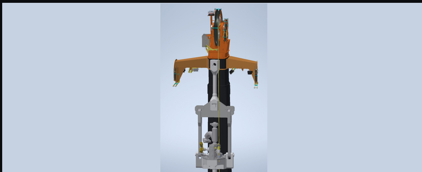
POWER SWIVEL AT WELL CENTRE – 12,500 FT-LB ROTARY TORQUE, DRIVEN BY THE ELECTRIC POWERTRAIN
