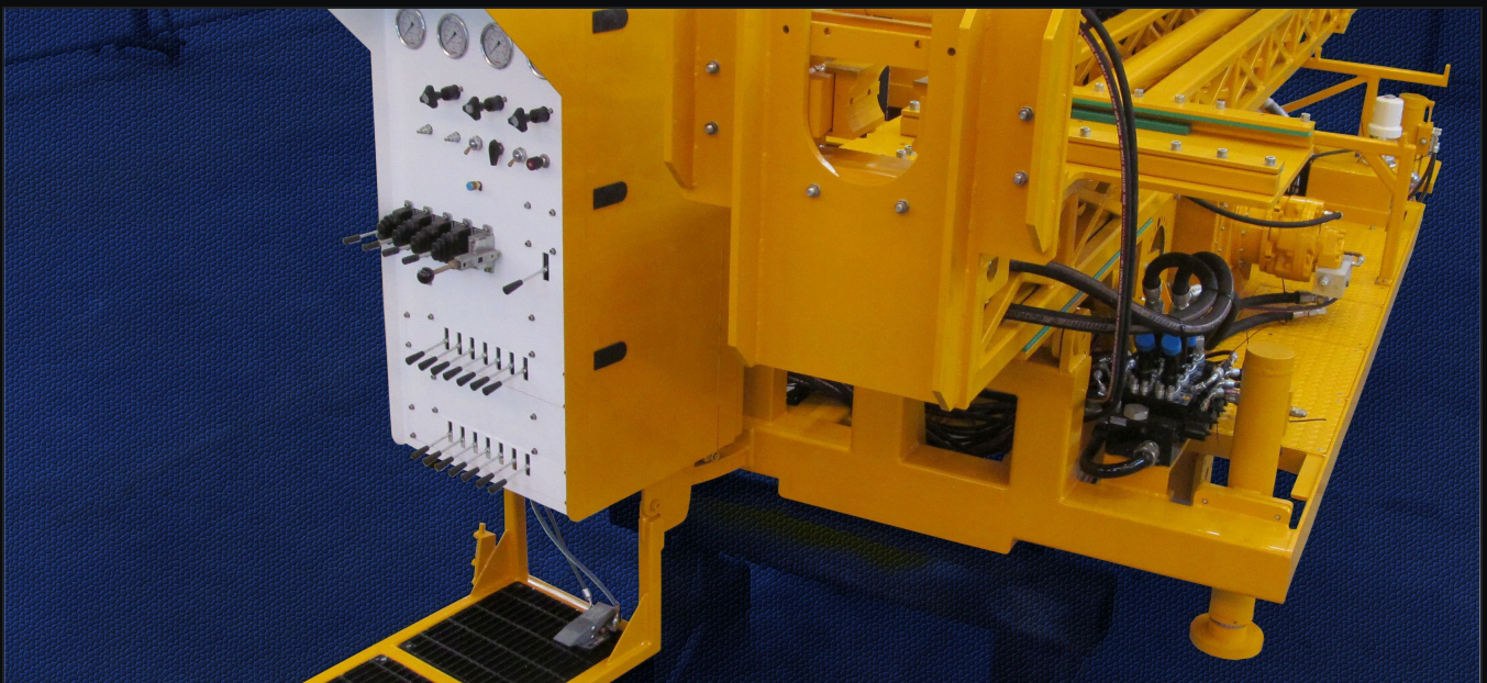
THE DRILLER'S PANEL ON THE DECK – GAUGES, LEVERS AND ENGINE CONTROLS IN ONE PLACE
