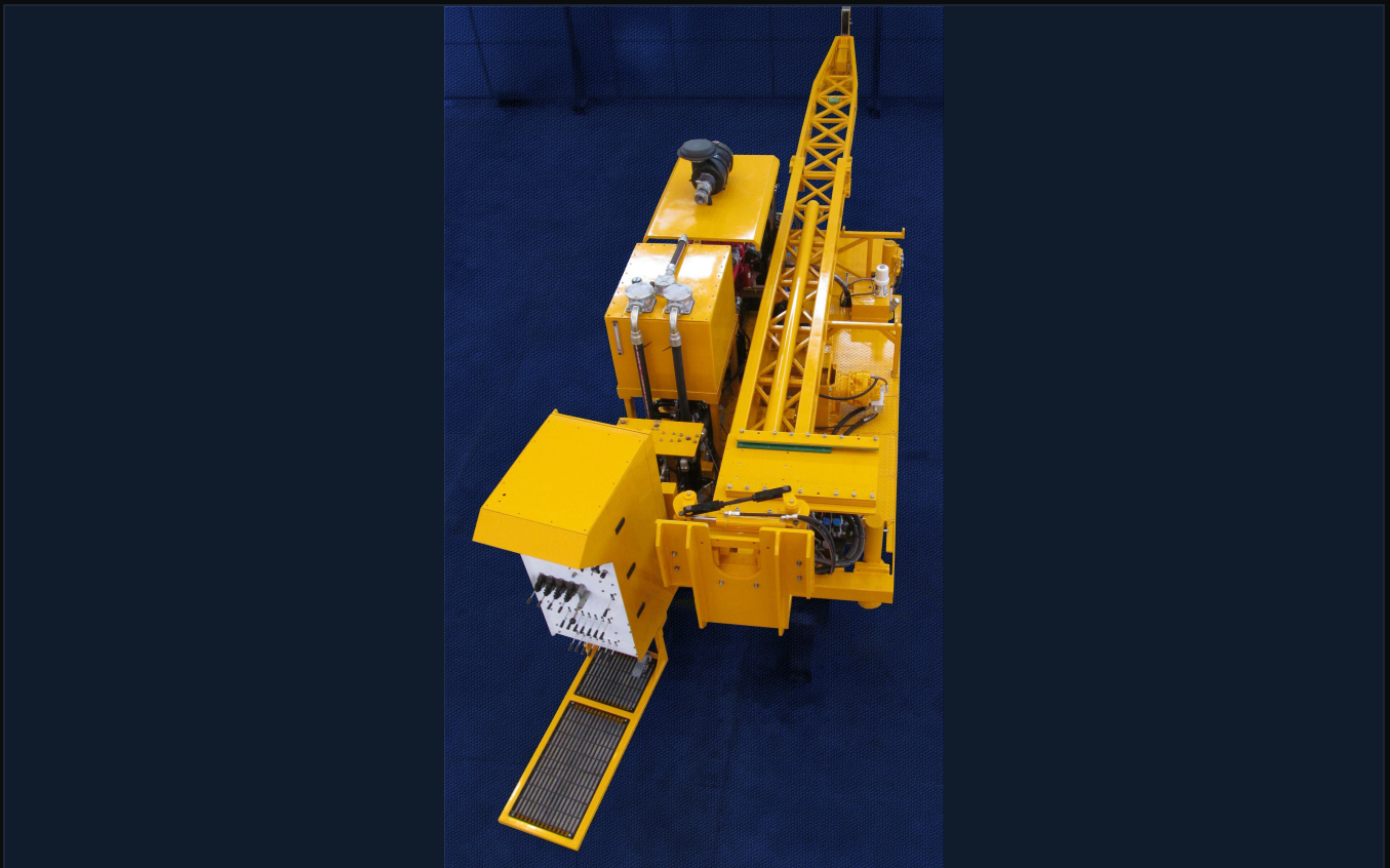
FOLDED DOWN ON THE DECK — MAST, HEAD AND FOOT CLAMPS STOWED INSIDE THE CONTAINER ENVELOPE
