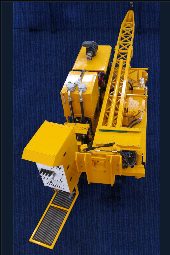
FOLDED DOWN – THE WHOLE RIG INSIDE A 20 FT CONTAINER ENVELOPE
