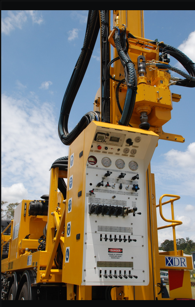
THE DRILLER'S CONTROL PANEL, SWUNG OUT TO THE WORKING POSITION
