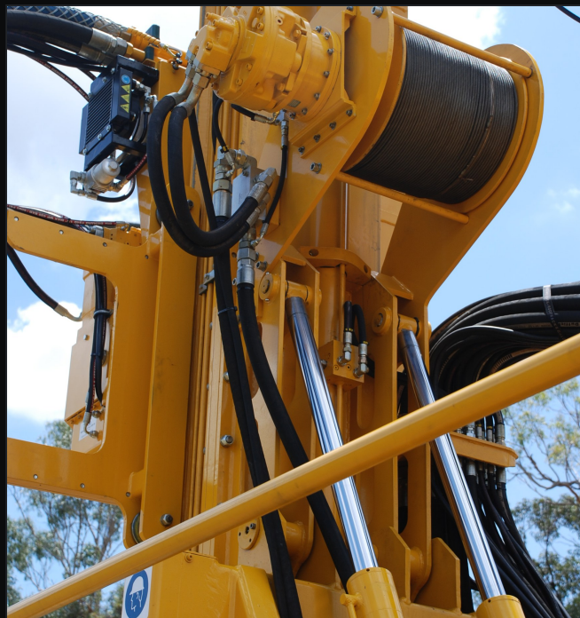
MAIN WINCH DRUM AND MAST HEAD – 16 MM NON-ROTATING ROPE
