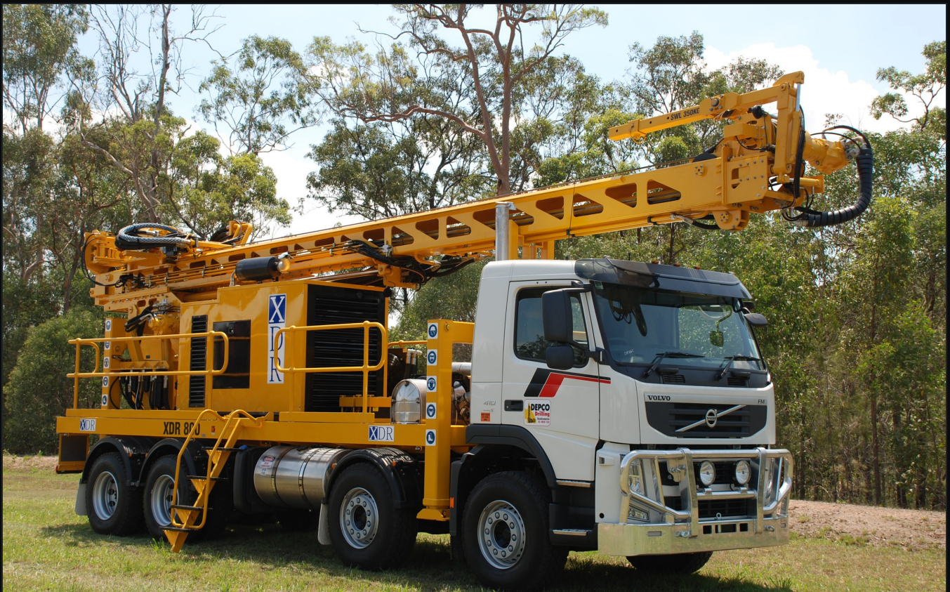
THE 800H ON SITE — 7 METRE DECK, MAST ERECTED, CONTROL PANEL SWUNG OUT
