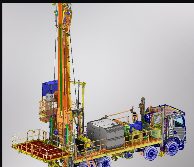
OPERATIONAL SETUP – MAST LUFFED, TELESOPED AND WEDGE-LOCKED
