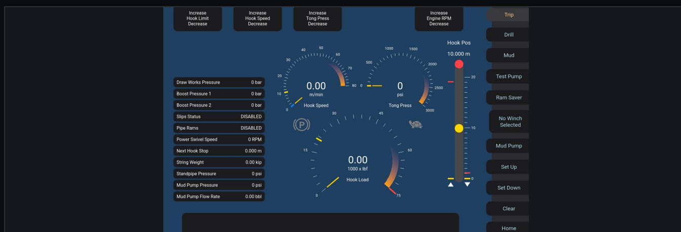
DRILLER'S HMI, TRIPPING SCREEN – HOOK SPEED, HOOK LOAD, TONG PRESSURE, HOOK POSITION AND STOP POINTS
