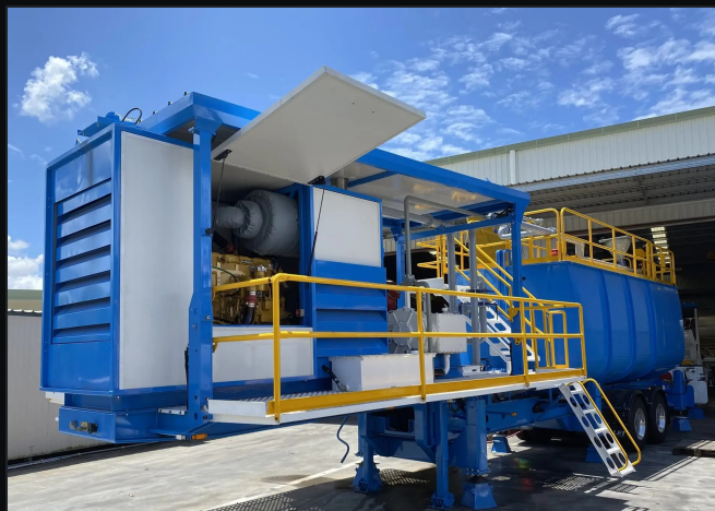
ENGINE ENCLOSURE AND DEPLOYED MAINTENANCE PLATFORM
