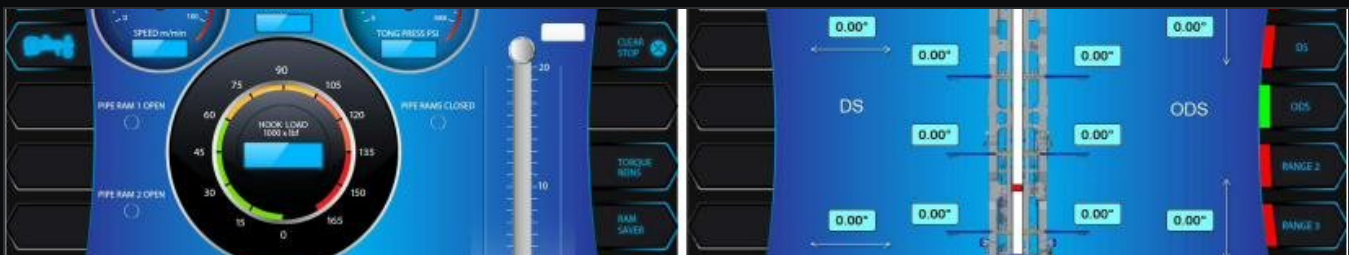
DRILLER'S HMI — HOOK LOAD, TORQUE, STANDPIPE AND TONG PRESSURE · CATWALK AND TROUGH POSITION
